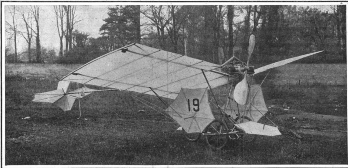
Three-Quarter Front View of the Aeroplane, Showing the Horizontal and Vertical Rudders in Front and the Combined Rudders at the Rear.
