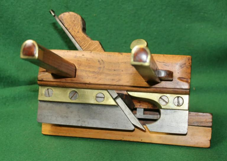
Lunnagan, NYC with owner name. NOTE: This maker is rated a 3 star \*\*\* in EMP Guide to American Wooden Planes. The cutter is marked Moulson Brothers Cast Steel Warranted No 4 and it measures: 8" L x 3/8" W. It is pitted but sharp. The slide arm wedges slide move easily and tighten properly. The brass turn screw and brass trim has been polished. The plane has a nice finish, feel and patina. It has NO issues...just a fine early plough plane
