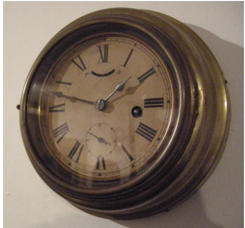
Picture 16: The US Clock Co timepiece with a 30 hour balance wheel movement, circa 1870. This clock was donated to the American Clock And Watch Museum in Bristol, CT by Harold B. Hubbell: Co-founder of THFHS and editor of the 1980 & 1995 History & Genealogy of the Hubbell Family
