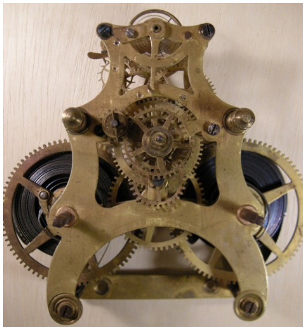
Picture 9: The Oct 10, 1865 design patent #2189 for a marine movement frame known as the “Christmas Tree” movement. This example has the balance wheel escapement.
