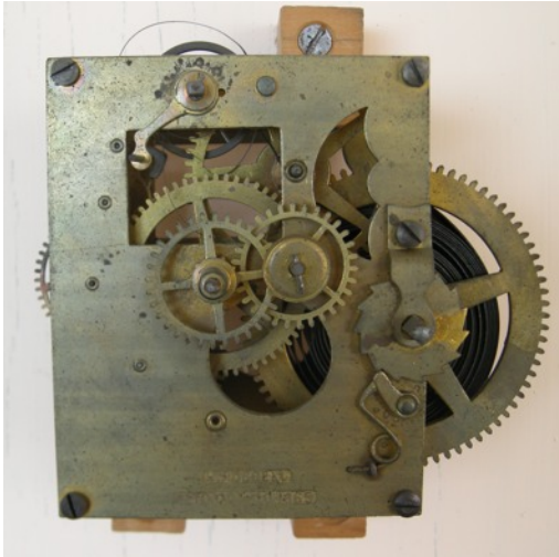
Figure 13: The “Unrella” movement developed around 1865. This example has the balance wheel excapement.
