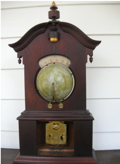
Figure 14: The Timby Solar Clock (left) with the front plate removed to show the movement, circa 1865 The Laporte Hubbell Solar Clock (right). Both clocks used Laporte’s “Unrella” movement with a balance wheel excapement.
