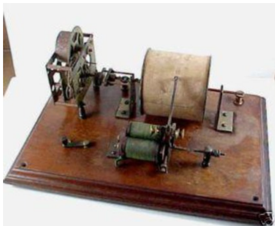
Picture 21: A telegraph register using Laporte's 30 hour balance wheel movement.
